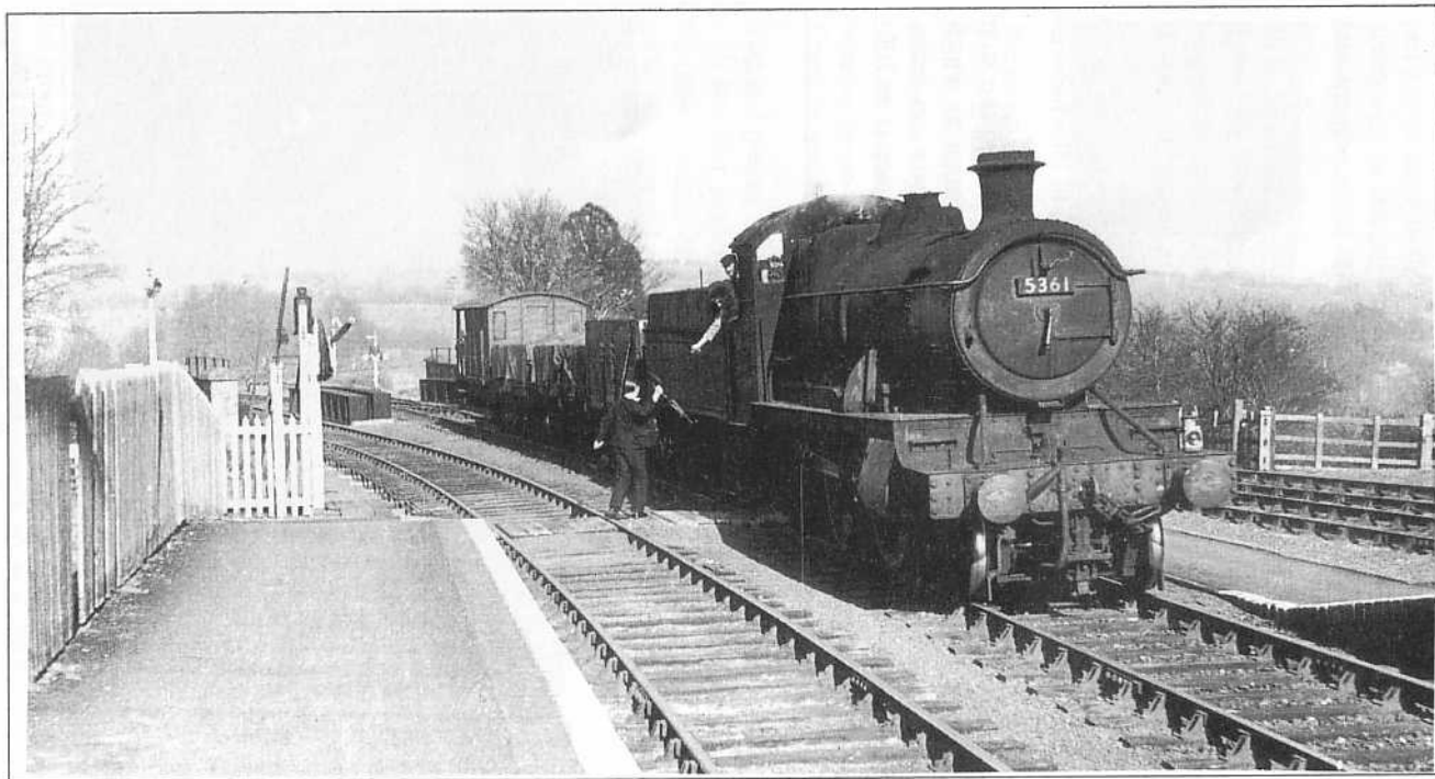
A very short 10.10am Banbury to Kingham goods arriving at Hook Norton behind the inevitable '43XX' class 2-6-0, in this instance Banbury's No. 5361, c.1950. This picture shows the signalman collecting the Bloxham section staff from the fireman as the train coasted gently towards the station, rather than having to walk to the set-down post at the opposite end of the station site. The crew on the engine may have been Engineman George Gardner and Fireman Tommy Burton, both of Banbury shed. Trains entering the running loops from the single line at Hook Norton were subject to a 25mph restriction, though that did usually trouble us unduly on the goods.
