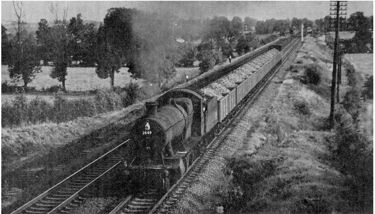
Fig. 9. A load of ironstone from the Oxfordshire Ironstone Company's quarries at Wroxton to South Wales by way of Fenny Compton, Stratford-upon-Avon and Honeybourne, is seen here on its way up Cropredy bank on July 31st 1961. The locomotive is an ex-G. W. R. 2-8-0 No.2849 of Newport (Mon.) shed, and the waggons are vacuum brake fitted tippers. Already this is an historic picture. The ironstone quarries are now closed, and steam engines are no longer to be seen in north Oxfordshire.
